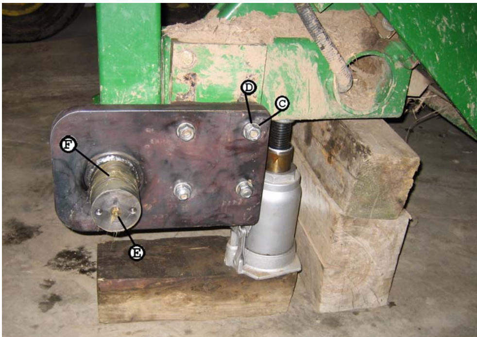
Figure 1. Pivot Plate Installation
